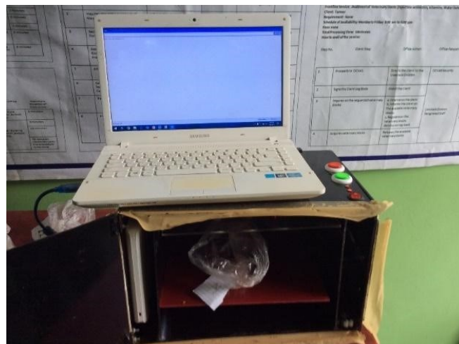
Figure 2. Actual data acquisition set-up for meat spoilage characterization.
