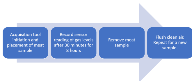
Figure 4. Workflow for the time-based measurement of the gas concentration levels and their rate of increase.
