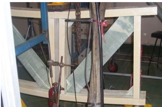
Figure 10. Modular composite truss panel [22]
