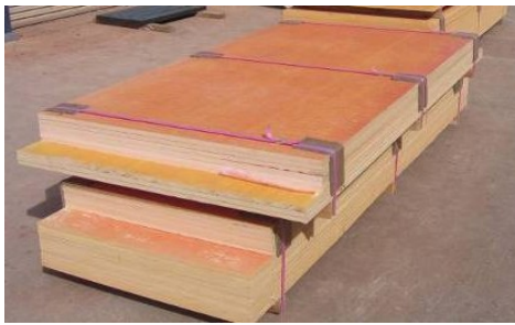
Figure 3. The novel fibre composite sandwich panel
