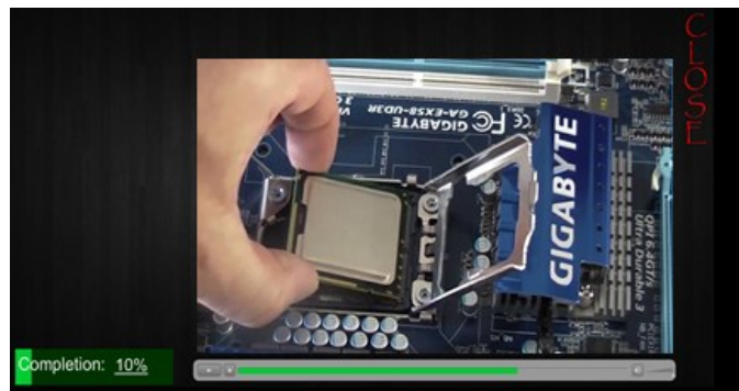
Figure 5. Video clip in installing motherboard components.
