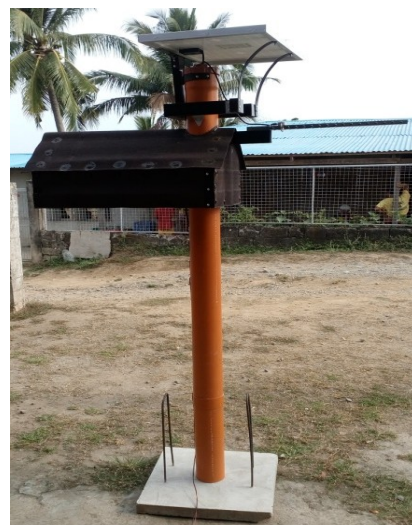
Figure 4. The Completed GEM device
