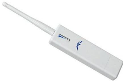
Figure 7. Wireless Router (Pico Station)
