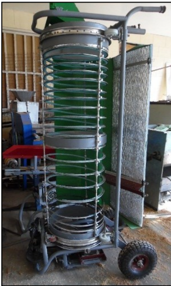
Figure 6. Potato grader in upright position
