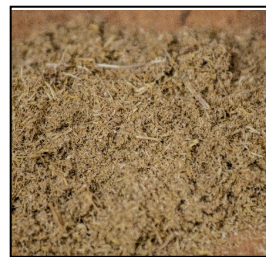
Figure 4. Banana fiber strands 1minute and double pass milled hammered
