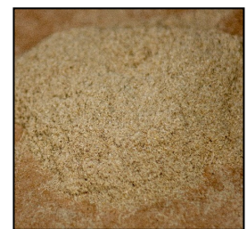
Figure 5. Banana micro-fibers through No. 40 sieve screened hammered
