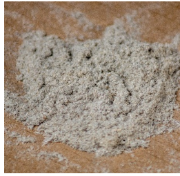
Figure 7. Rice straw micro-fibers screened through No. 40 sieve
