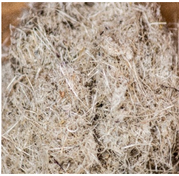
Figure 6. Rice straw hammered 1 minute and double pass milled
